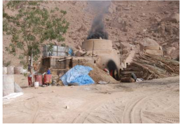
Fig. 18-2 A kiln of mud bricks.
