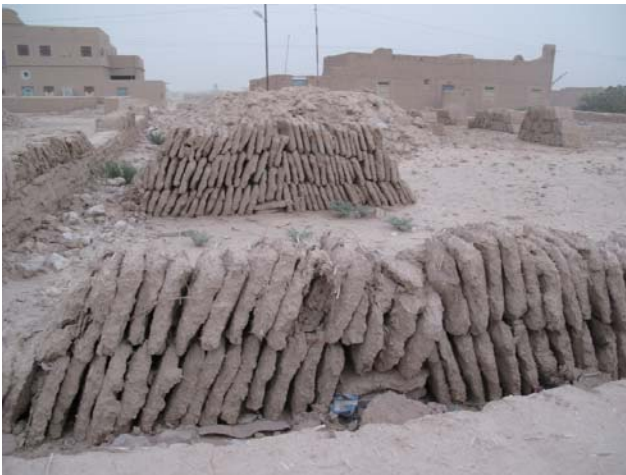
Fig. 4-3 Bor , piled-up mud bricks in the remains of houses.
