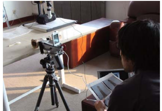
Measurement with a portable X-ray fluorescence analyzer
