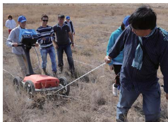
Practical training of ground penetrating radar (GPR) survey at the Boralдай burial mounds (Kazakhstan)
