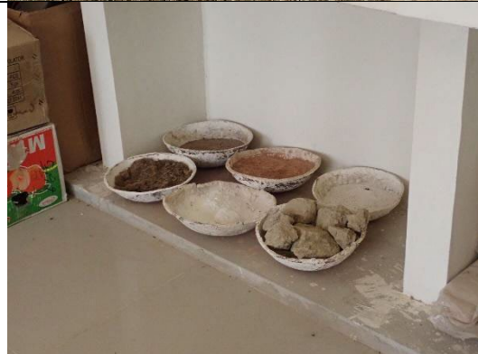
Fig.7 Mixing tests of adhesives with gypsum as the main ingredient. Experiments with various soils.
