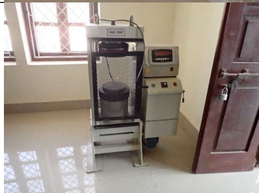
Fig.8 Strength tester for measuring the strength of adhesives. Compressive strength is used as an indicator.
